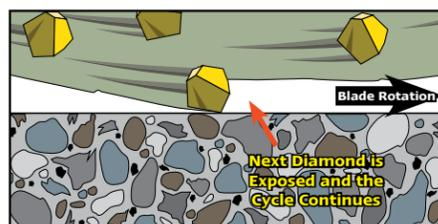
As the old diamonds are fractured and worn away they are replaced by new diamonds and the process continues until the segments are worn down to the core.
