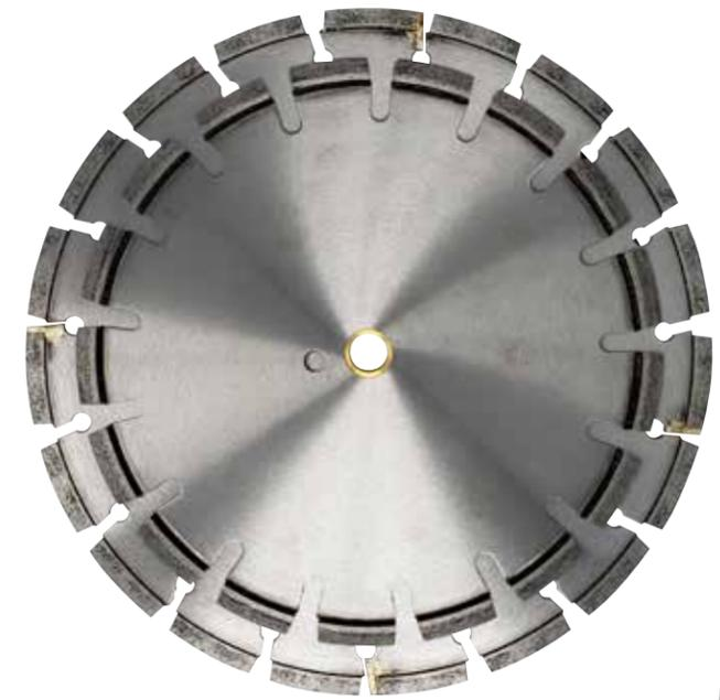
WDS bevel blades are used to cut a bevel angle when cutting joints. Creates a V-Cut. Each blade has a 45 degree angle, leaving a 90 degree bevel in the cut when used in a two blade stacked configuration. These blades are sold as a matched set of 3 blades. A center line blade, and 2- 45 degree angle blades.
